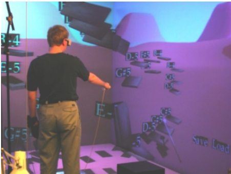
Figure 2. A performer playing the Virtual Xylophone. By moving and creating new plates, the performer has created a custom interface for playing a particular musical piece.
