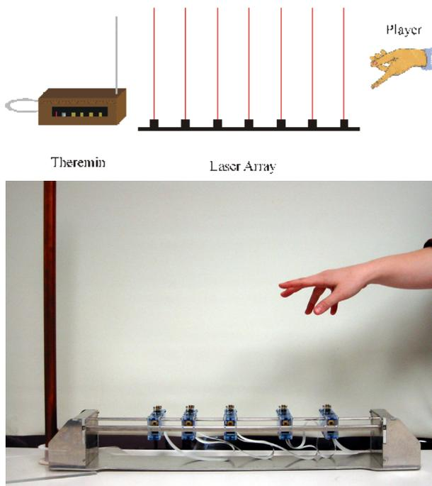
**Figure 1: System Diagram (above) and as built (below)**
