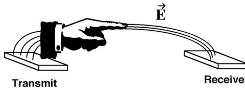
Figure 4: Capacitive Transmit Mode
