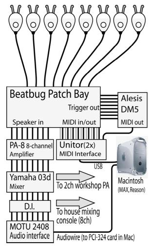
Figure 2. Beatbug rack schematic.
