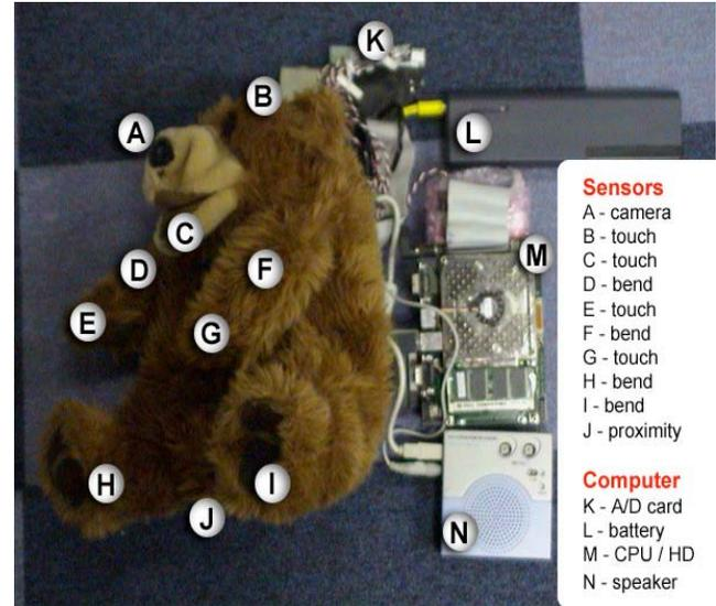
Figure 2. Hardware components.
