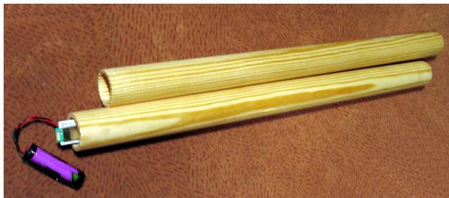
**Figure 3. Complete Aobachi interface (battery and Bluetooth® module shown for scale).**
