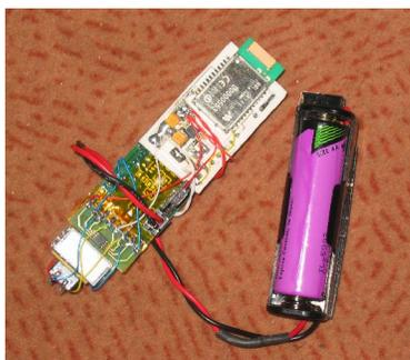
**Figure 2. Aobachi embedded hardware powered by a AA size battery.**
