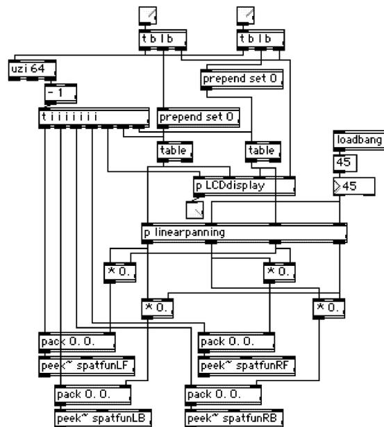
**Figure 5:** The four-channel version of the subpatch that converts two sets of *multiSlider* values into amplitude coefficients for four spatial information tables. The linear panning subpatch contains two copies of the stereo panning algorithm, the output of which is cross-multiplied to generate the four amplitude coefficients for localizing a monophonic sound in quadrasonic space.
