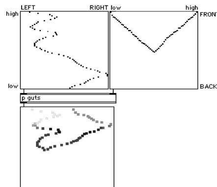
**Figure 4:** A spectral spatializer controller using separate *multiSlider* objects for left-right and front-back localization. The *lcd* display indicates the location of FFT energy bins in two-dimensional space. Color is used to indicate the relative frequency of each bin.
