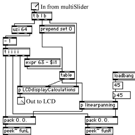
**Figure 2:** A subpatch showing conversion from the *multiSlider* controller to twin spatial information tables. The speaker-to-speaker panning subpatch is borrowed directly from the MSP panning tutorial.
