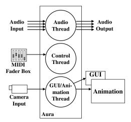
Figure 1. System configuration for The Watercourse Way.
