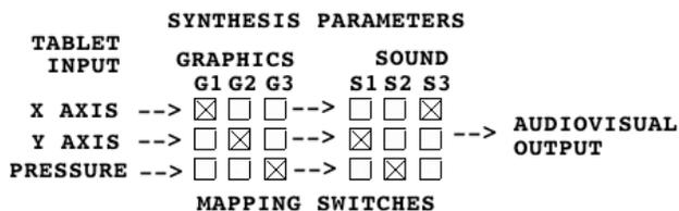
Figure 1: *Miró*'s mapping mechanism.
