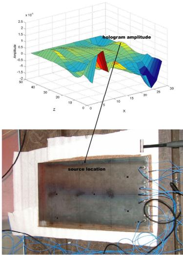
**Figure 5.** Measurement on a metal-plate and associated amplitude distribution.
