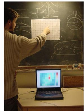
Figure 4. Touch detection experiment with Time Reversal.
