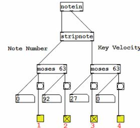
Figure 7. Pd patch for quadrant decoding.
