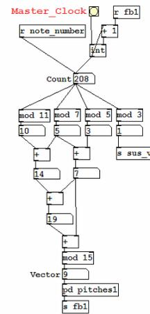
Figure 8. Pd patch for cyclic sequence generator.
