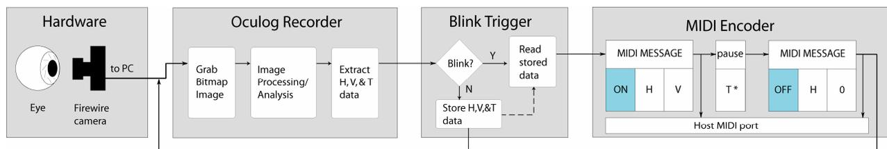
**Figure 4. Overview of Oculog eye movement system.**
