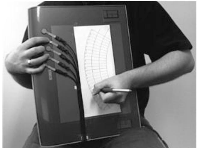
Figure 1: Representation of the "HandSketch" controller in use : Wacom™ tablet, with radial pen diagram, and 8 FSRs (Force Sensing Resistors).
