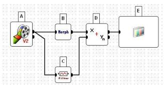
Figure 3: blocks B and C are executed in parallel, on separate CPUs if more than one is available. Data is resynchronized before being sent to block D.
