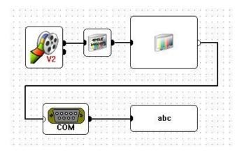
Figure 2: A clock signal is generated by a VideoDisplay, and is used to synchronize a serial input block
