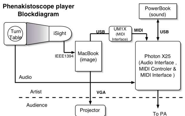
Figure 1. Blockdiagram of “Phenakistoscope player”
