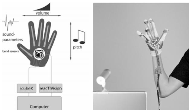
Figure 3. VRemin II – Hand tracking and Glove (prototype)
