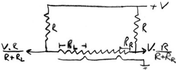
Figure 2 Sensing 2 points with Membrane potentiometers
