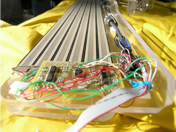
**Figure 5: Stringless Cello Position and Pressure Strips**
