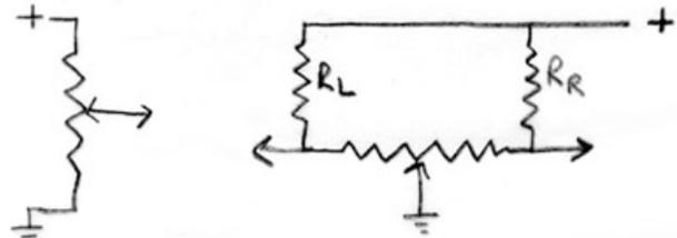
Figure 1. Potential divider (left), and Grounded wiper (right)
