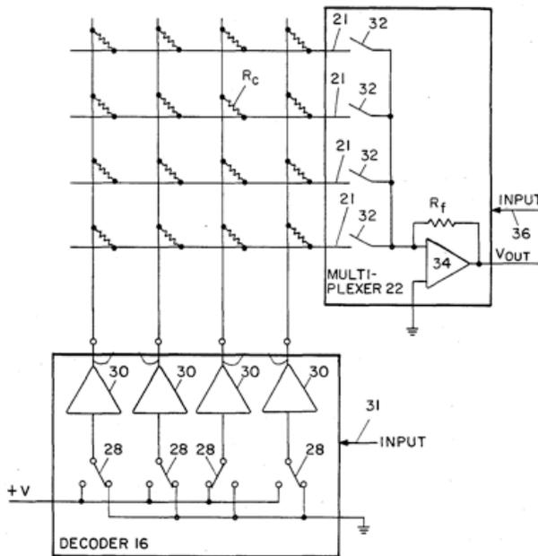
Figure 12 Grounding and virtual ground sensor isolation
