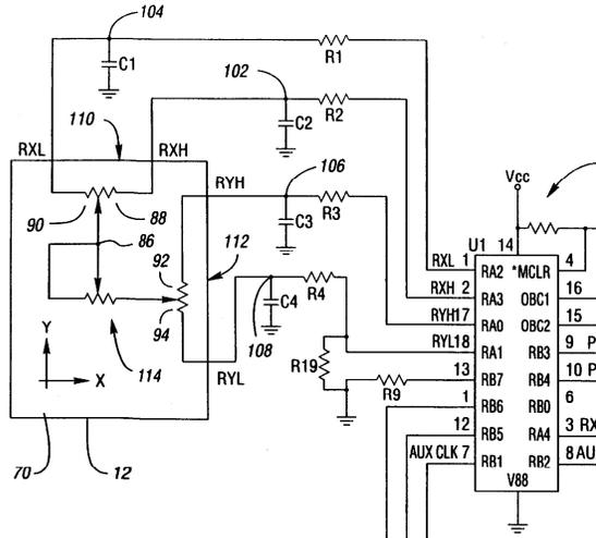
Figure 9 Interlink Versapad Scanning
