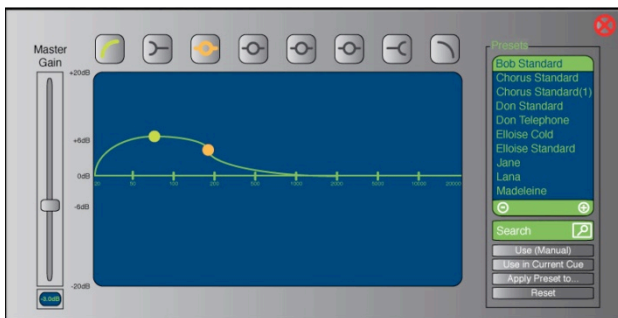
Figure 4. Cuebert multitouch equalizer
