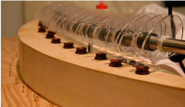
Figure 3. Rose Wood Bridges Transfer The Vibrations
