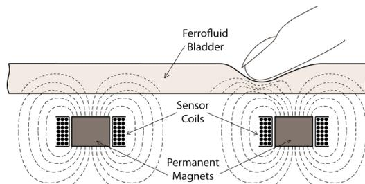
**Figure 2. Cross section through sensor coils, showing disturbances to the magnetic field.**
