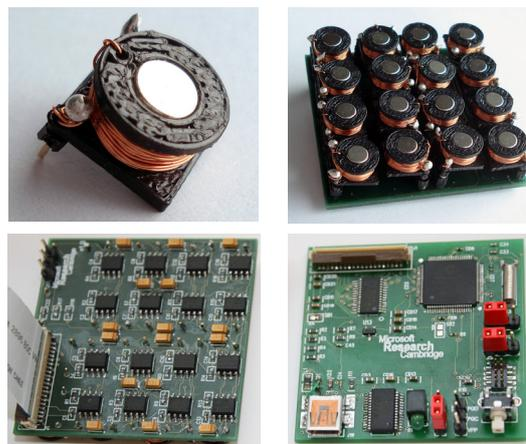
**Figure 3. (i) Individual sensor coil, (ii) 16 sensor coils mounted on the reverse of the analogue board, (iii) analogue sensing board, (iv) digital interface board.**
