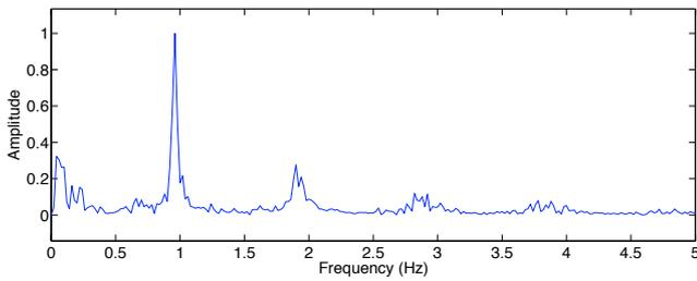
Figure 2: Spectrum of typical PPG Signal
