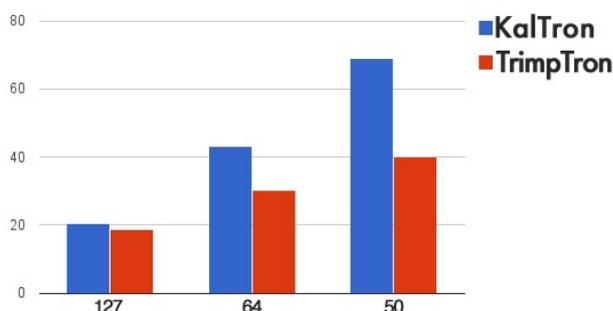
Figure 5. Actuator Speed Tests (X-axis = MIDI velocity; Y-axis = Strikes/Second)
