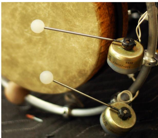
Figure 2. TrimpTron Solenoids
