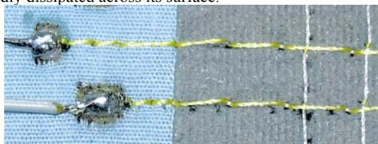
Figure 8 Soldered thread
