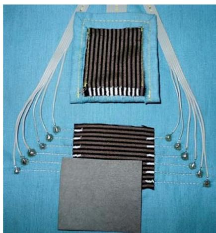
Figure 5: Strain-relieved cabling and solder pad
