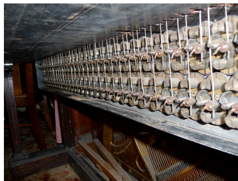
Figure 1. Solenoids from a Tel-Electric system installed under the keys of an Ivers & Pond upright piano
