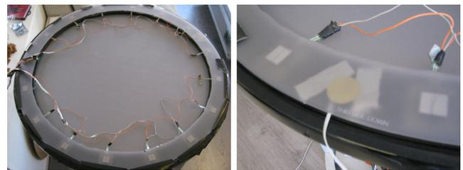
Figure 1: A top view of the tabletop annulus. On the right a detail of the contact microphone.
