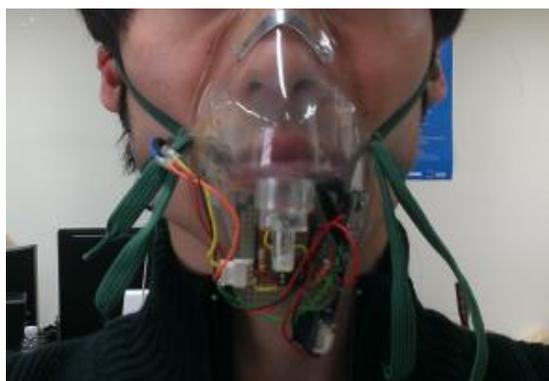
Figure 1. Respiration sensor device
