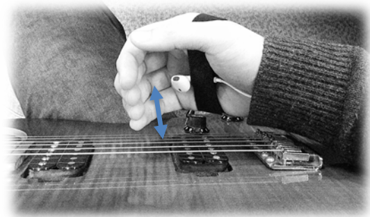
Figure 3. Transmitter and receiver (earphone and pickup)
