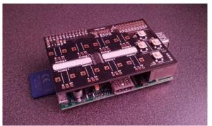
Figure 2. Raspberry Pi with a LOP shield (NOP variant).
