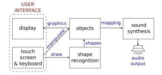
Figure 1: The user interacts with a touch screen display and a keyboard to draw new shapes on to the screen and manipulate existing ones. New shapes are processed by the shape recognition module that identifies what type of instrument or effect the sketch represents. Once an object's type has been decided, it can be played, moved, resized or deleted by the user. The musical synthesis engine generates the sound associated with an object when it is tapped.
