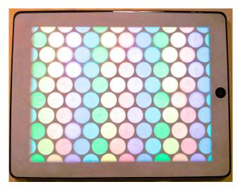
Figure 2: Haptic feedback iPad overlay.
