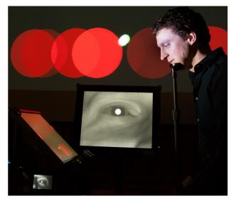
Figure 5. The display components used in *EyeMusic v1.0*. The audience and the performer each see a large view of the control surface, and a small video feed of the eye image.
