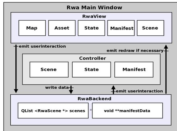
Figure 2. Communication diagram for the RWA-Creator
