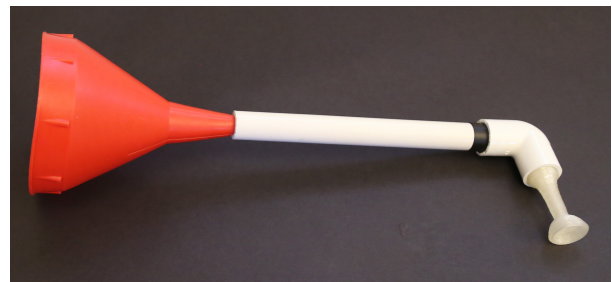
Figure 2. A “Trumpet” made with PVC middle section and a “Bell” made of an oil funnel.
