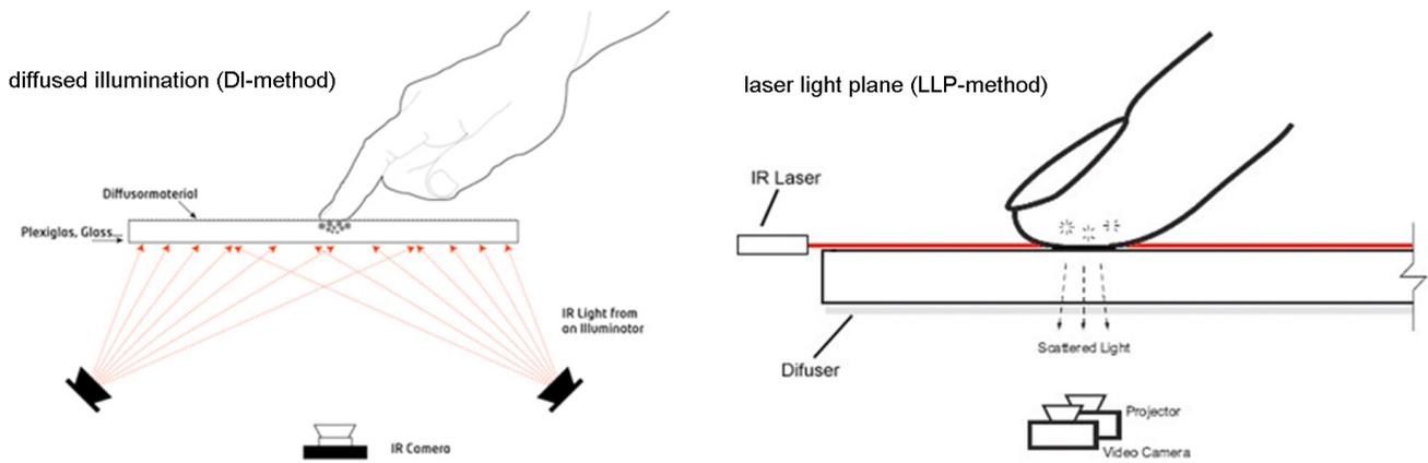
Figure 2: IR-Illumination for the optical finger-tracking. [Graphic-source: wiki.nuigroup.com/hardware]
