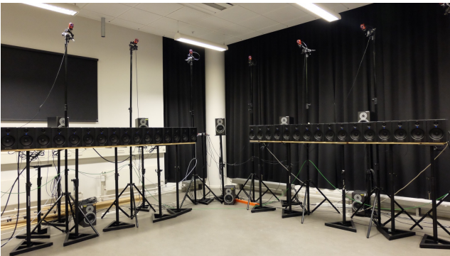
Figure 1: The playing area surrounded by the WFS arrays and OptiTrack Motion Capture system.
