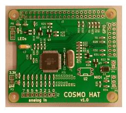
Figure 2: COSMO-HAT circuit board to connect 8 analogue controller inputs, 8 LED's or switches and MIDI I/O.
