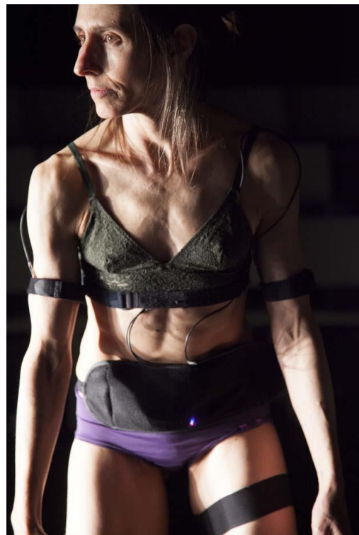
Figure 1. Each Emovere performer had three EMG sensors positioned in the left and right biceps, and in one quadriceps, as well as one ECG sensor positioned in the torso.
