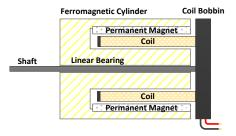
Figure 1. VCA Cutaway.
