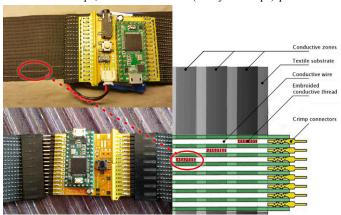
Figure 5: Bus system – Schematic representation (right) and example of ribbon sewn to PCB (left, top) and ribbon crimped to female headers (left, bottom). Connections are made by sewing conductive thread where ribbon and strips overlap (highlighted in red)
