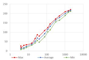
Figure 7: Weight (x-axis, grams) vs sensor output (y-axis)
