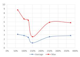
Figure 9 – Pressure point size (x, in percent of strip width) vs absolute error in two-dimensions (y, in mm).
