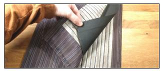
Figure 3: Multi-layer structure of eTextile sensor: nonconductive (outside), piezo resistive (center) and conductive (in strips) materials combine to form the sensor.
