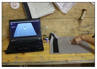
Figure 2: eTextile sensor based on the design described in this paper. Visualization provided by host application.
