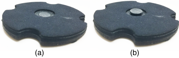
Figure 4: A percussion pad that attaches on top of MM-RT. A custom 3D printed solenoid is attached in the center of the pad. (a) A solenoid at rest. (b) A solenoid actuated.
