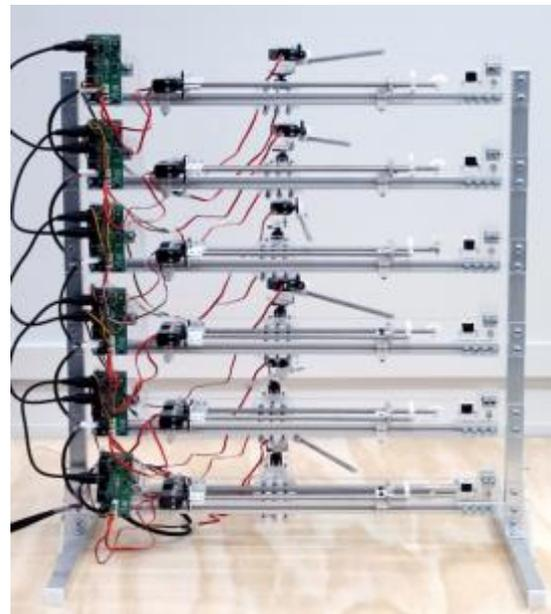
**Figure 1. *Swivel 2*, a parametrically rich mechatronic chordophone.**
