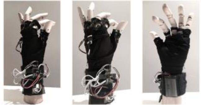
**Figure 4. *g.qin*, a gestural controller that measures the metacarpophalangeal joint's range of motion (ROM) of all fingers (except the little finger) and the wrist, together with linear acceleration of the instrumentalist's left hand.**
