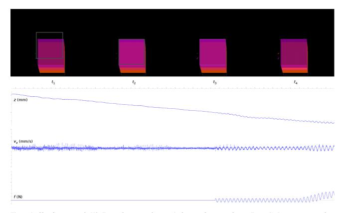
**Figure 4** Ghostfinger example I/O. Top: right-eye visual output (to be viewed at an angle: see Figure 3). Bottom: corresponding position input, speed input, and force output, occurring along the z axis over time.
