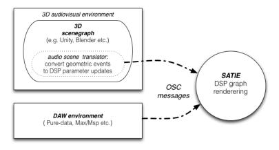
Figure 2: OSC messages control sound object parameters (individually or by group) at different levels. For controlling SATIE, 3D scenegraph can convert geometric events to lower level spatializer parameters. Geometry-related computation can be added to SATIE though the use of mappers than can provide higher level parameter control, such as for DAW environment.
