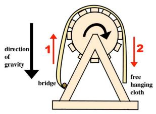
Figure 3: Diagram of the two-part rotational gesture afforded by the acoustic wind machine in a clockwise motion, and the difference in the cloth tension on each side.
