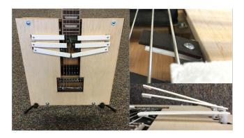
Figure 1: a) Full instrument, b) Damper, c) Hammer
