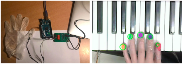
Figure 2: The force sensor glove and Image recognition using RGB camera
