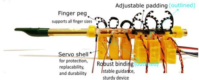
Figure 5. The overall design of flute device.
