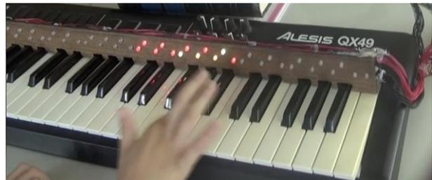
Figure 1. MIDI controller mounted with a LED stripe.
