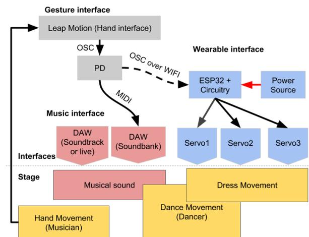
**Figure 2. Schematic diagram of the interfaces, internal systems and components and stage elements. Red blocks represent the structure of musical interfaces. Blue blocks represent mechanical interfaces. Yellow blocks represent elements that involve movement.**
