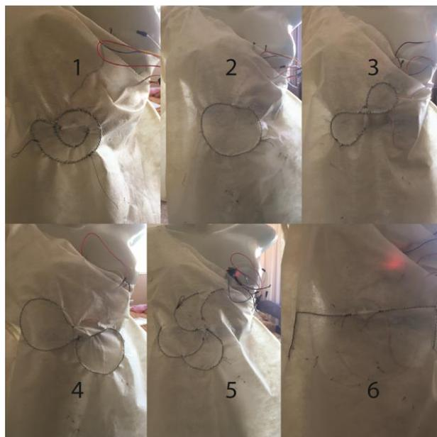
**Figure 3. Test structures with the Servo Motor. Structure 1: spiral, structure 2: circle, structure 3: Möbius small, structure 4: Möbius large, structure 5: radial, structure 6: line.**
