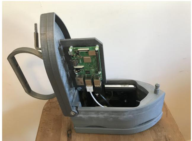
Figure 4: Interior of iron: showing Pi, battery, Arduino, and USB audio interfaces.
