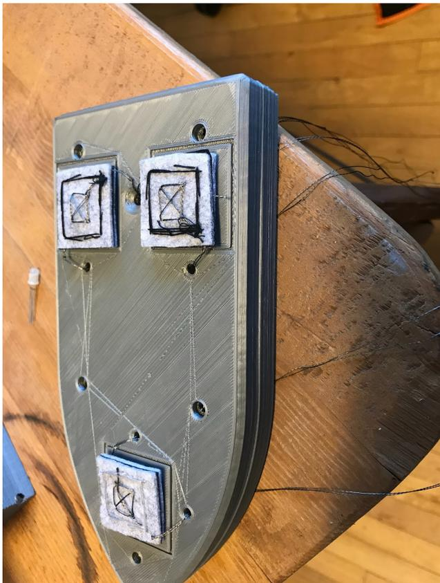
Figure 3: Pressure Sensor Assembly in-progress
