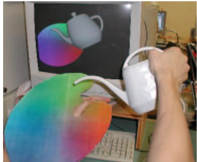
Figure 1: MetaMuse is controlled by two props: a watering can and a palette.
