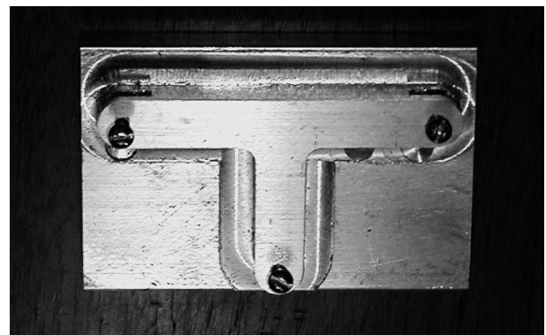
Figure 4: Fixturing the T-part for CNC machining
